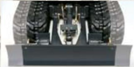
With the simple removal of one pin, its quick-fold blade adjusts in size instantly.
